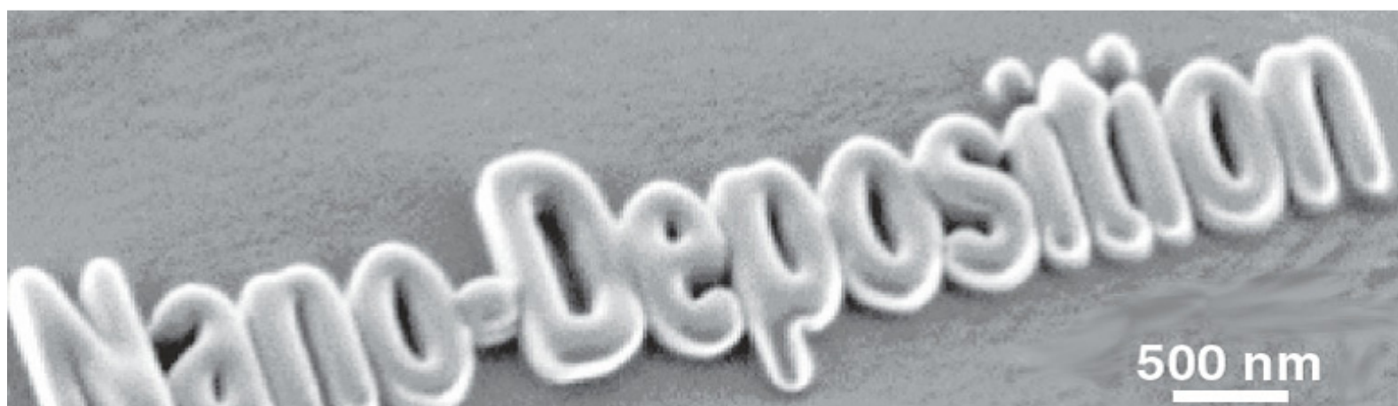
Figure 1: FIB deposition results which have good resolution and material range but low deposition rate.
